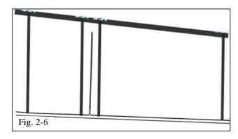
(h) Trim the excess length on the vertical pieces of tape beyond the tape installed in Step 3(g) (Fig. 2-6).
