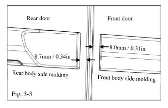
(c) Align the rear edge of the front molding with the vertical mark on the tape located 8.0mm (0.3 in) forward of the rear edge of the front door (Fig. 3-3).
