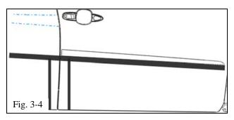
(d) Align the bottom of the front molding flush with the top edge of the tape spanning the doors (Fig. 3-4).
