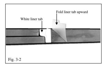
(b) Remove white liner tab and fold the adjacent liner tab upward at the front end of the molding such that the tabs are accessible during install (Fig. 3-2).
